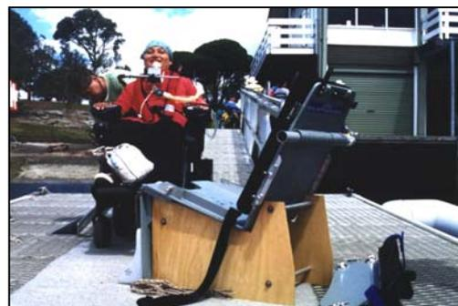
2. Set up the sailing seat on its stand correctly positioned beneath the transferring hoist. Open both or one of the arm rests and one or both the shoulder supports, clear the shoulder straps making ready for the transfer.
