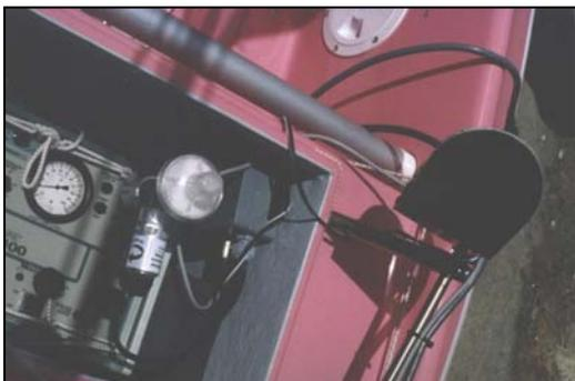
7. Pass the chin operated panic switch and strobe light leads through the 1" hole behind the sailors right shoulder and plug them into the safety circuit control box.
