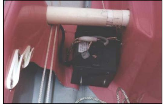
The batteries supply the ventilator and also power a strobe light (located on the seat backrest) which will operate at all times during normal ventilator function. The strobe light plugs into the control box which is in turn connected to the batteries and the ventilator alarm circuit. The strobe light stops operating in the event of a ventilator alarm.
